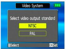
The video output signal can be switched to NTSC or PAL to accommodate different regional standards. The appropriate setting will vary between regions.
